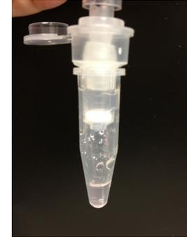
Centrifuge the Burst cartridge to break the film and collect directly into your collection tube or vial. Fewer steps and no risk of contaminating your sample with the pellet.
